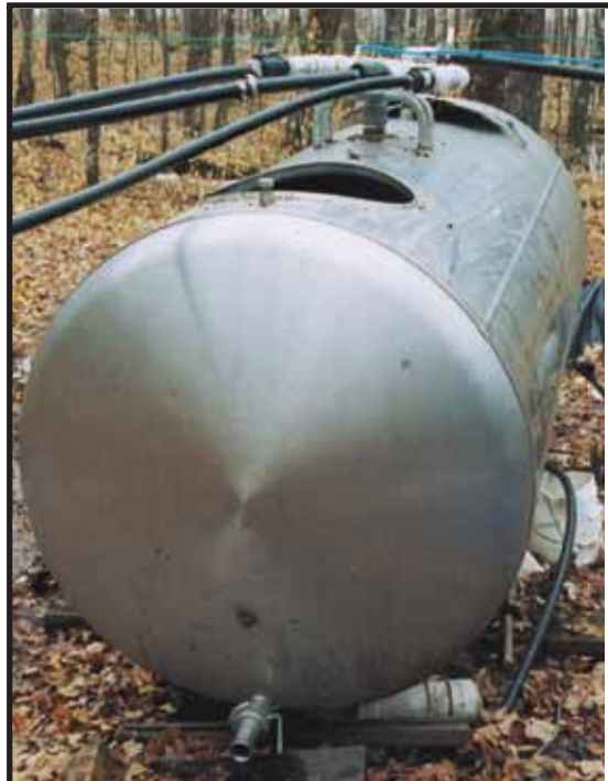
Gravity carries the sap through the tubes to the storage tank. From the storage tank, a vacuum pump feeds the sap into a large evaporating trough housed in a covered processing shed.
