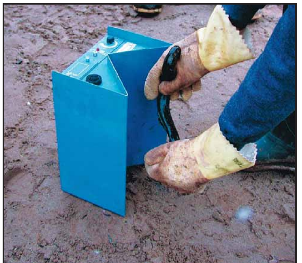
GLIFWC fishery aides pass lamprey over a U.S. Fish & Wildlife Service coded wire tag reader to determine the presence of an embedded tag.
