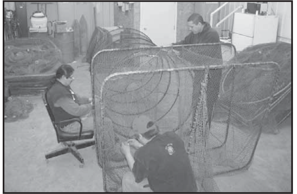
Another view of fyke net repair in GLIFWC's garage. Ed White, fisheries technician, along with Kris Arbuckle and Josh Johnson, both inland fisheries aides, tackle a fyke net from all sides, basically busy sewing up holes and tears. (Photo by Butch Mieloszyk)
