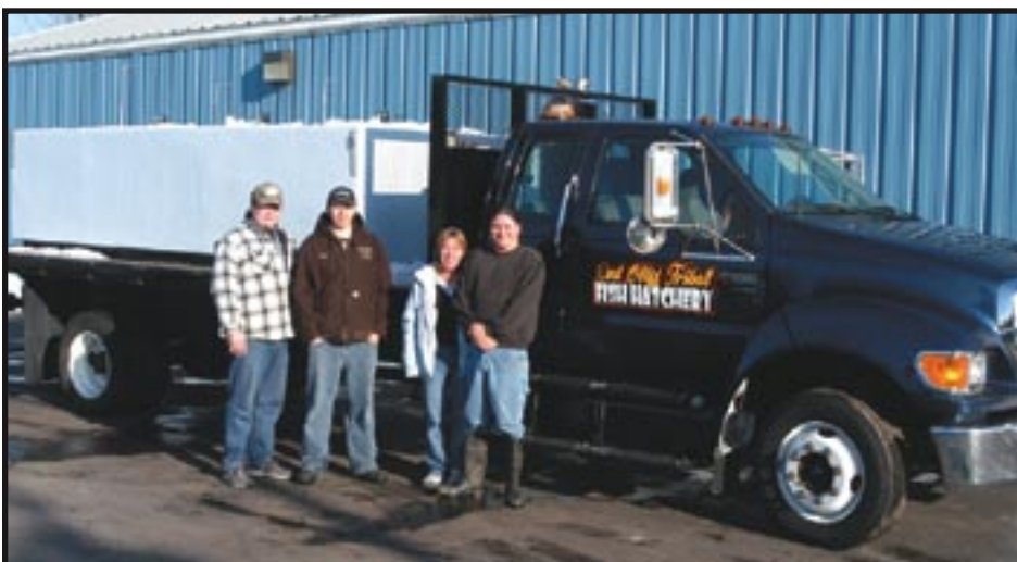
A new hatchery truck fitted with with a 900 gallon tank can transport everything from fingerlings to five-year-old fish. Purchased with assistance from a Bureau of Indian Affairs grant, Red Cliff hatchery staff will utilize the vehicle to transport fish like coaster brook trout hundreds of miles for stocking in public waters and private ponds. Pictured are technicians Daryl Boyd and Brian Bainbridge; Office Manager Shelly Gurnoe and Hatchery Manager Sean Charette. (Photo by Charlie Otto Rasmussen)
