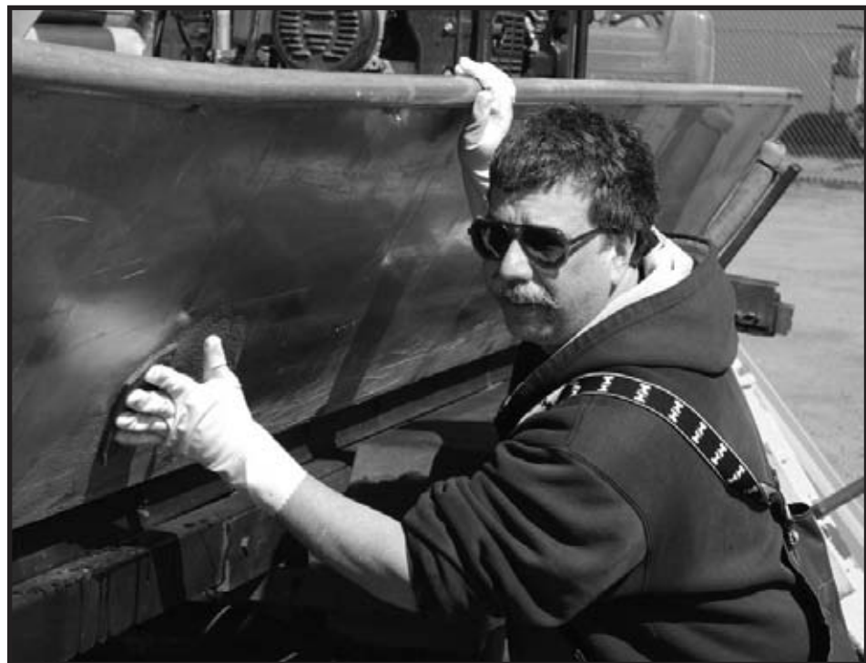
Time for clean-up after a busy spring season. Crew Leader Butch Mieloszyk cleans off an oxide build up that accumulates on the hull of the shocking boats. If left, the oxide layers impede the electroshocking mechanisms of the boat. (Photo by Sue Erickson.)
