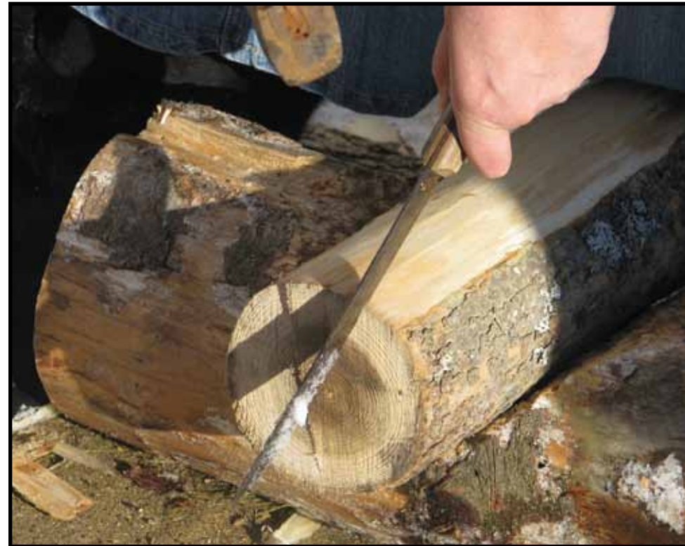
The black ash log is being scored to determine the width of the growth ring that will be lifted.
