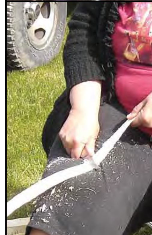
With the flat rounded edge of the axe, every inch of the strip is pounded at least two times.
