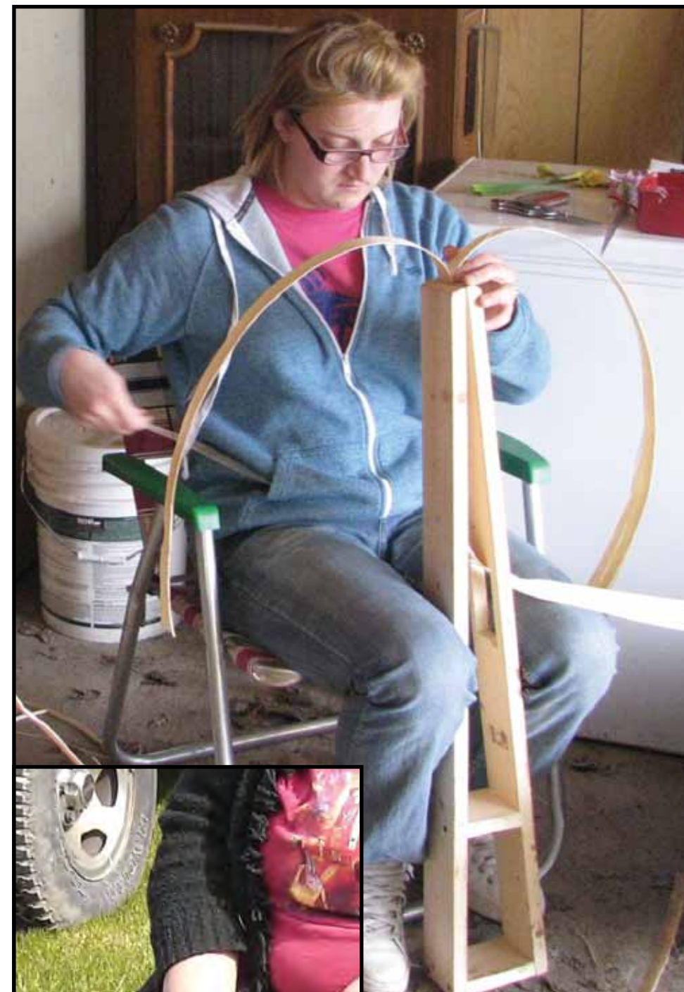
Upper photo: Strips are separated and each put into a "splitter." The top of the strip is scored halfway across with a knife and the strip is pulled up and outward, splitting the growth ring down the middle. These are called splints.
