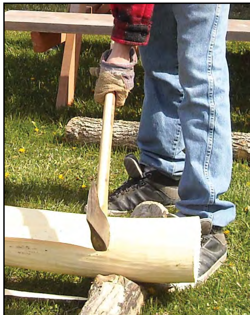
With the flat rounded edge of the axe, every inch of the strip is pounded at least two times.
