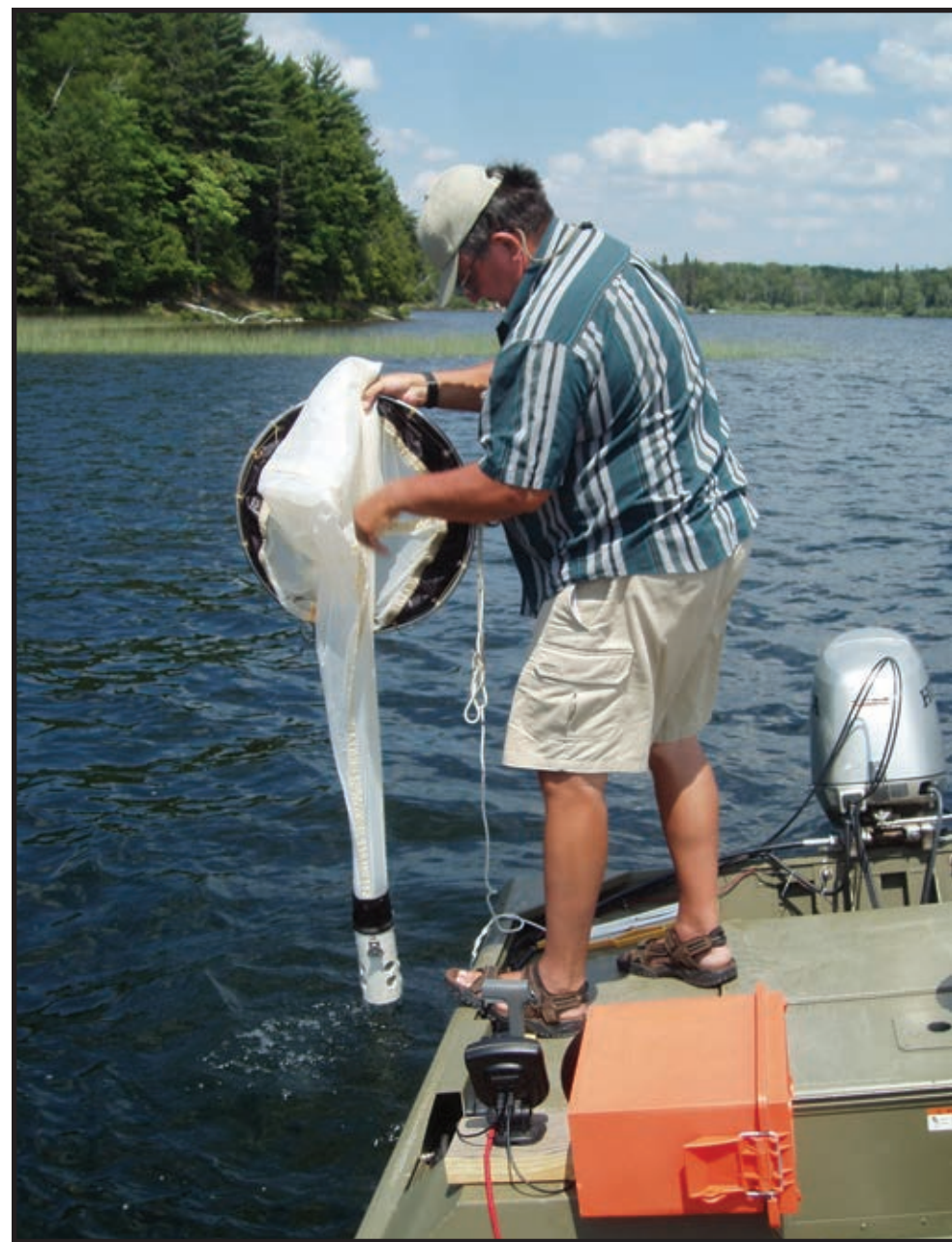
GLIFWC performs annual surveys of ceded territory lakes, checking for the presence of aquatic invasive species, such as zebra mussels, spiny waterfleas, and Eurasian water milfoil. When sampling, the location is marked by GPS and noted. Later samples are shipped to a laboratory for identification of invasive species in the sample. Above Sam Quagon, a member of GLIFWC's aquatic invasive species crew, prepares to drop a veliger net, checking for the presence of zebra mussel veligers. (Photo by Dara Olson)
