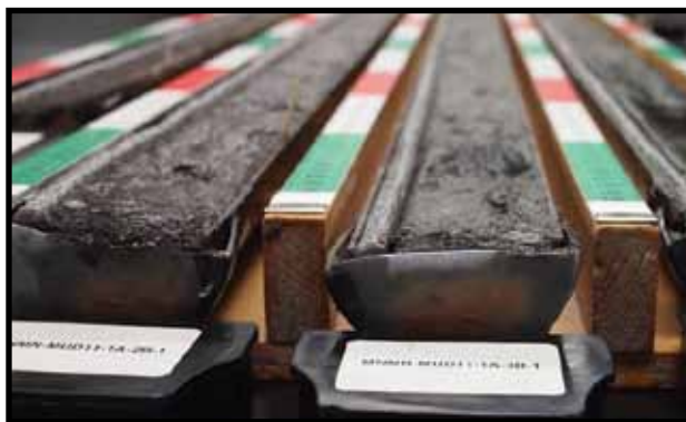
Bisected core samples from Fond du Lac Reservation's Mud Lake. (Photo by T. Howes)
