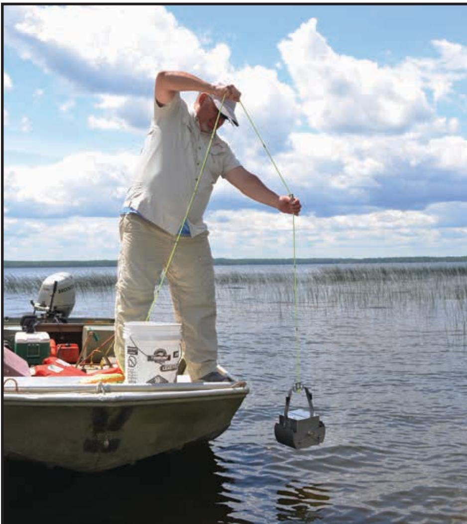
Resource Specialist Sam Quagon lowers an Ekman dredge into Lake Lac Vieux Desert's Misery Bay, part of a multi-lake GLIFWC effort to detect the aquatic invasive species, spiny water fleas. The spring-loaded dredge collects a 6x6" sample of silt, which is being analyzed by laboratory technicians. (COR)
