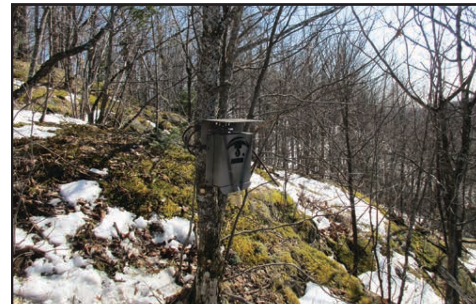
Time-lapse camera used to monitor tree canopy phenology at one of the GLIFWC phenology study sites. (Hannah Panci photo)
