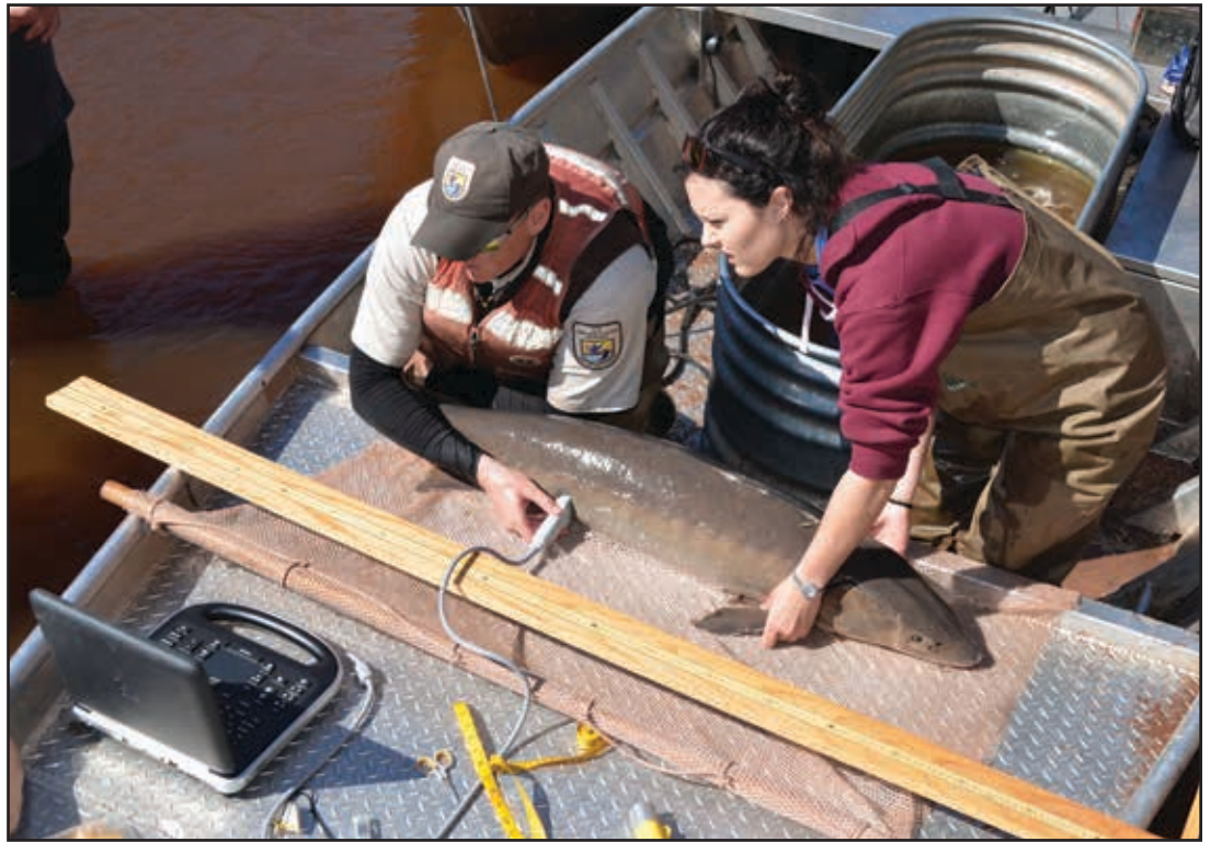
Portable ultrasound equipment allows fisheries biologists to determine the sex of lake sturgeon. (COR)
