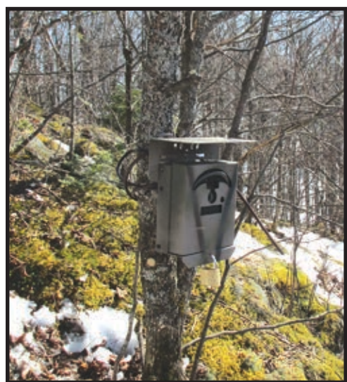
Figure 1. Photo of a phenocam at one of the GLIFWC phenology study sites. The phenocams are placed in a sturdy metal security box in an attempt to keep bears and other curious animals from disturbing or altering the view of the camera throughout the growing season.
