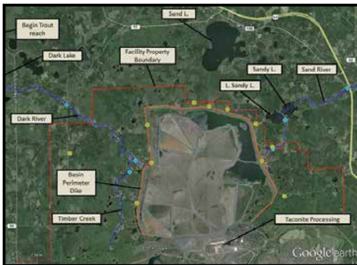
Figure 1. The lakes and rivers receiving discharge water from the Minntac tailings basin. The primary receiving waters are the Sandy and Dark Rivers. (Map courtesy of the Minnesota Pollution Control Agency)
