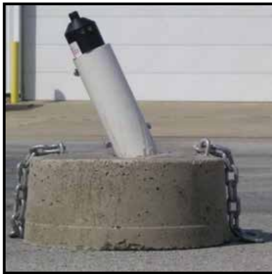
Image 2. An acoustic receiver attached to a mooring. Receivers will be positioned throughout the lake. (Dr. Chris Vandergoot photo).
