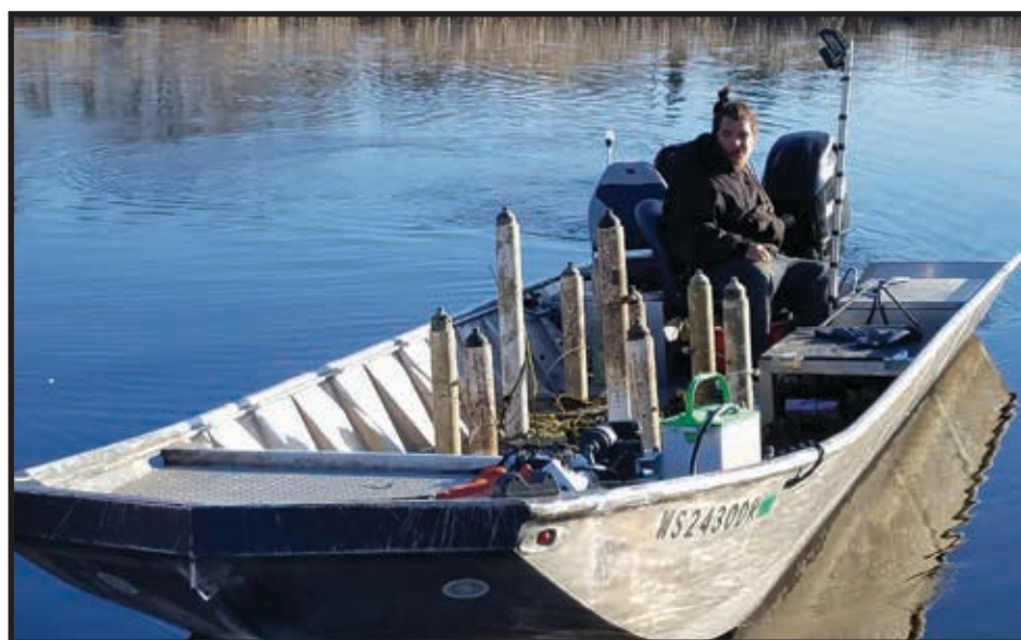
Acoustic receivers appear lined up aboard a survey boat. Biologists studying the Mille Lacs Lake fishery submerged individual receivers down to the lake bed, creating a grid to track the movements of fish that have been implanted with a transmitter. (A. Shultz photo)
