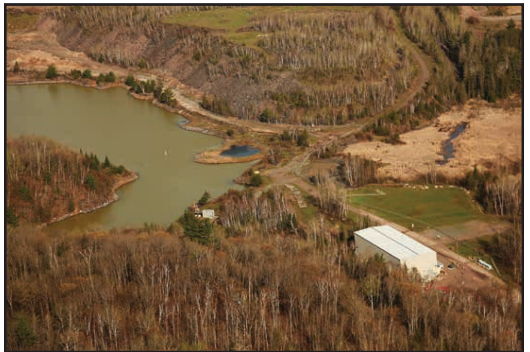
Photo 1. Wastewater treatment plant and flooded historical iron mining pit. Waste water from the ore processing plant at the south end of the pit lake (off left of photo) is discharged into the pit lake, treated by the wastewater treatment plant and discharged to wetlands or, more recently, directly to the Escanaba River (off right of the photo). C. Moran photo)
