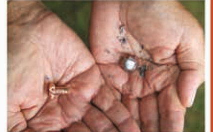
A copper bullet on the left and a lead bullet on the right after a shooting demonstration. (Photo: Paul A. Scott / Milwaukee Journal Sentinel)
