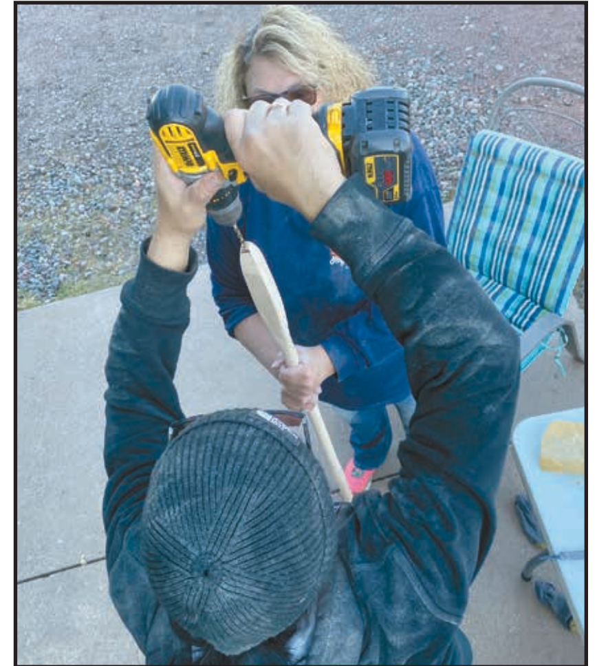
Lynn Plucinski steadies a goonikaa-ginebig as Minogizhig drills a hole that will hold pewter, adding weight to the head. (COR)
