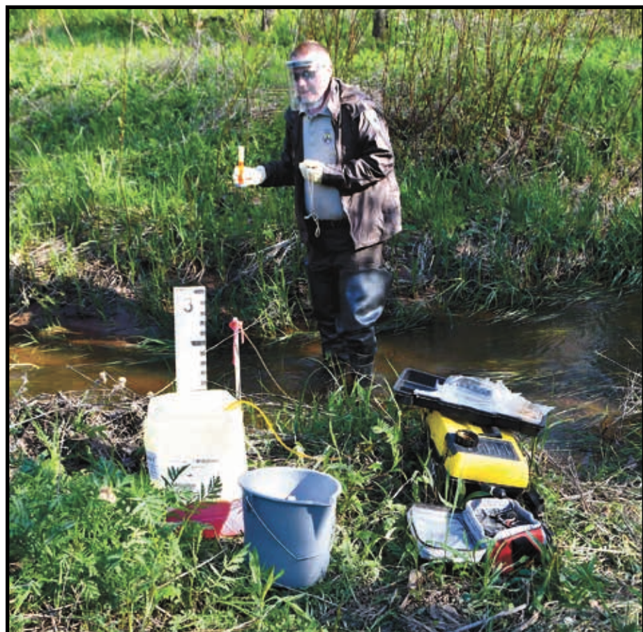
A US Fish & Wildlife Service technician monitors the infusion of the lampricide TFM into a Gichigami tributary. TFM targets larval lamprey before they develop into parasitic adults. (CO Rasmussen photo)
