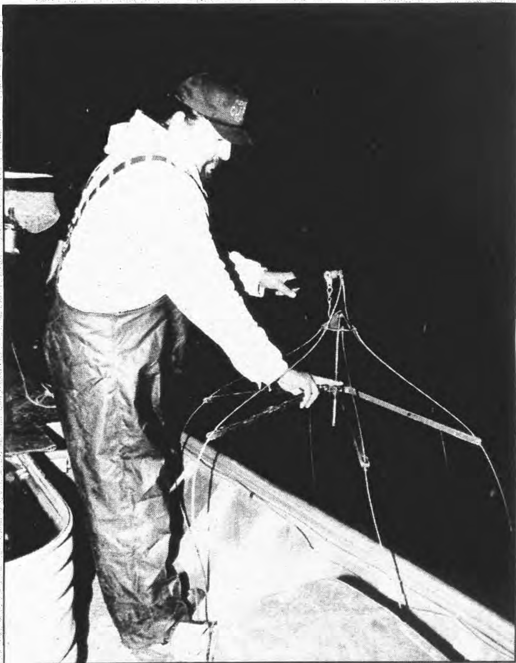
Mitch Soulier retracts one of the two shocking booms before an electrofishing run on Siskiwit Lake, Bayfield County. The booms are mounted off the bow and pass an electrical pulse into the water that briefly immobilizes fish. Along with Ed White, Soulier is an 11-year veteran of GLIFWC inland fisheries electrofishing surveys. (Photo by Charlie Otto Rasmussen)
