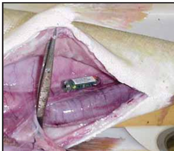
Above is one of the tags recovered from a lake trout. Each tag holds up to 37,000 records of depth and temperature. (Photo courtesy of Shawn Sitar, MiDNR)
