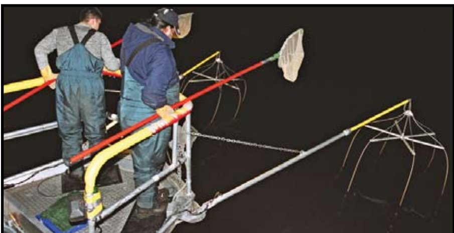
A GLIFWC electrofishing boat cruises the shoreline of Parent Lake in Upper Michigan. (Photo by Charlie Otto Rasmussen)
