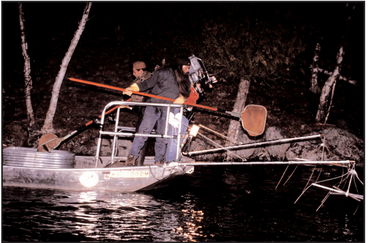
This is an electrofishing boat used for fish population surveys. Those arms that reach off the bow of the boat with spider-like things on the end put a low-volt shock into the water and slightly stun the fish. The crew then scoop the fish out of the water to be counted, measured, sexed, and then returned to the lake.
