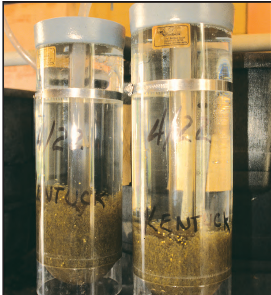
These are Bell jars used in hatcheries to incubate fish eggs, in this case walleye eggs from Kentucky Lake. Once hatched, the little baby fish, called fry, are either stocked back into a lake or reared in the hatchery to a larger size called a fingerling.
