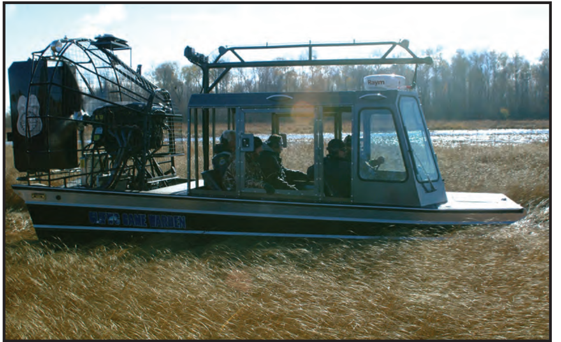
A new airboat became part of the GLIFWC Enforcement Division's arsenal of rescue equipment this fall. Manufactured by Diamondback Airboats in Florida, the 24-ft. boat is capable of going on land, water and ice, and can reach speeds over 50 miles-per-hour on ice. Four GLIFWC officers participated in a three-day training that was part of the purchase deal. Trained officers include Dan North, Tom Kroplin, Steve Amsler, and Jim Stone. Currently, at the GLIFWC main office in Odanah, Wisconsin, the airboat is mobile and available on an as-needed basis 24 hours, round the clock. (photo submitted)
