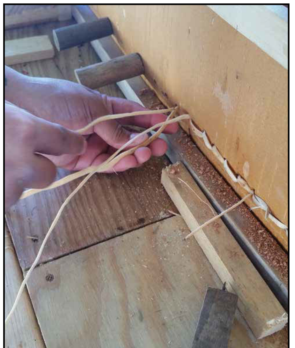
The bark is sewn together using holes drilled in the wiigwaas one inch apart.
