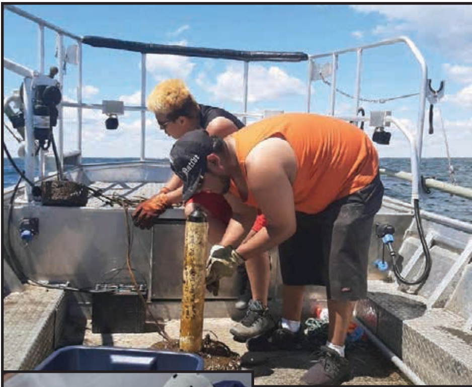
Mille Lacs Band fisheries staff retrieve receivers from Mille Lacs Lake to download fish detection data, replace batteries, and inspect the units for damage. The receivers are then placed back into the lake to collect additional data.
