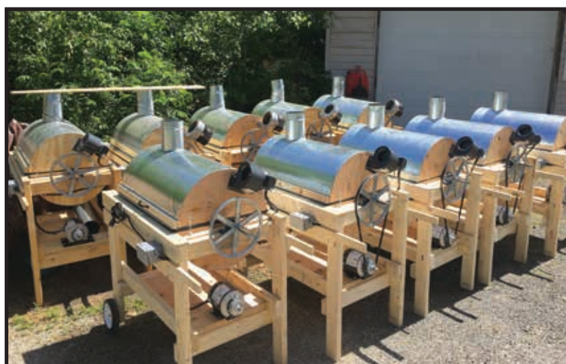
Manoomin threshers were built for GLIFWC-member communities. These machines can thresh 400 pounds of rice in two hours. (D. Bruyere photo)
