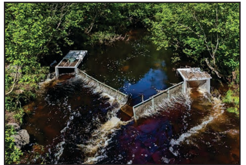
KBIC's Natural Resources Department staff continue to set, monitor, and maintain supplemental control traps in seven streams around the Keweenaw Peninsula. Through the supplemental control research project, a new style of adult assessment trap was set at the Traverse River (pictured), where previously fyke nets had been fished.
