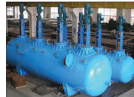
Beneficiation equipment: autoclave for hydrometallurgy.
