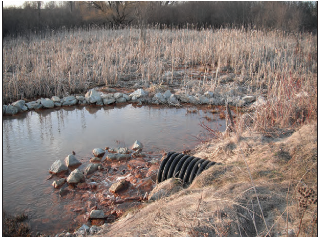
Acid rock drainage at the Buck and Dover mine in Michigan. The water flows into the Iron River.
