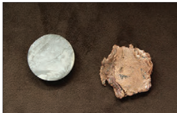
Comparison of a disseminated copper ore (left) and a piece of native copper (right). Disseminated ore bodies have a small amount of metallic mineral by volume.
