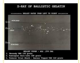
Image shows lead fragments which are distributed throughout the ballistic gelatin, varying in size from large to microscopic.
