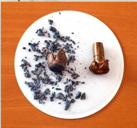
The difference between a lead ammunition (pictured on the left) and a nontoxic copper ammunition (pictured on right) seen in the picture above.
