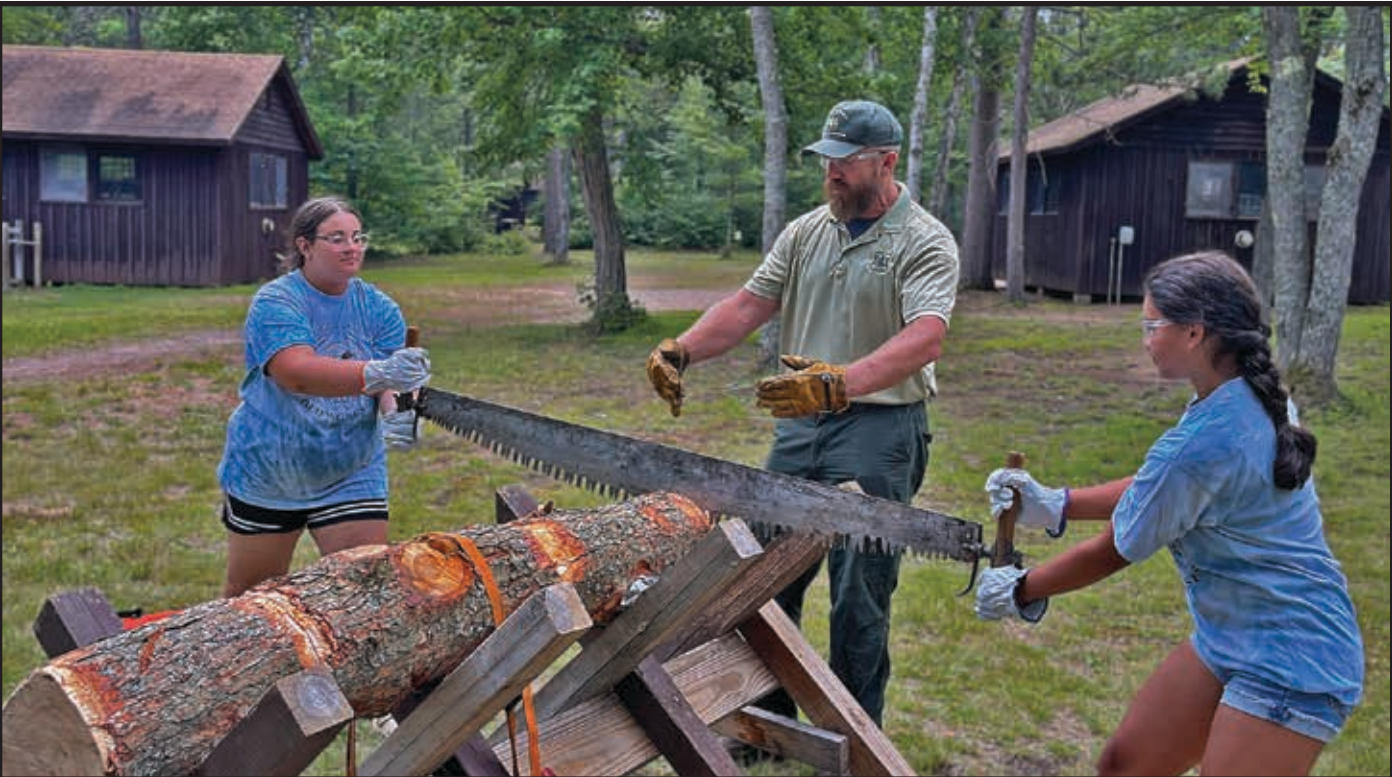
Campers learn how to use a manual crosscut saw from Aaron Woof, USFS. Crosscuts are used for trail building and maintenance where chainsaws are not allowed. (JVS photo)
